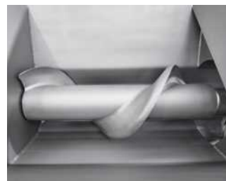
Infeed hopper shown from top view
