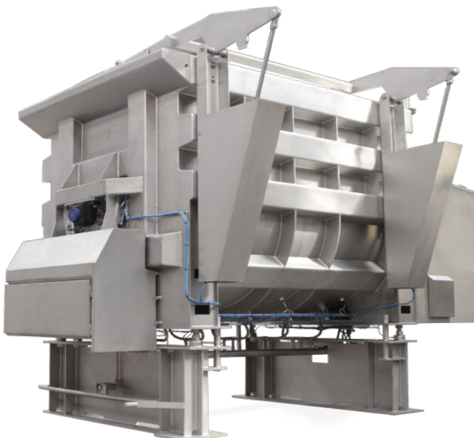
scansteel foodtech® scanDefrost 10.000 L with view of steam injection system
