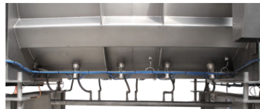
scansteel foodtech® scanDefrost 10.000 L with view of steam injection system
