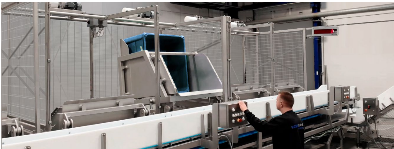
One option in the scansteel foodtech® "batching family of solutions" is a station of typically 2 – 8 swing loaders (tippers) which can hold different meat raw material.
