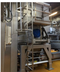
Final installation of Whole Pallet Crusher, WPC 2000-Single, at customer site, shown with platform with ladder.
