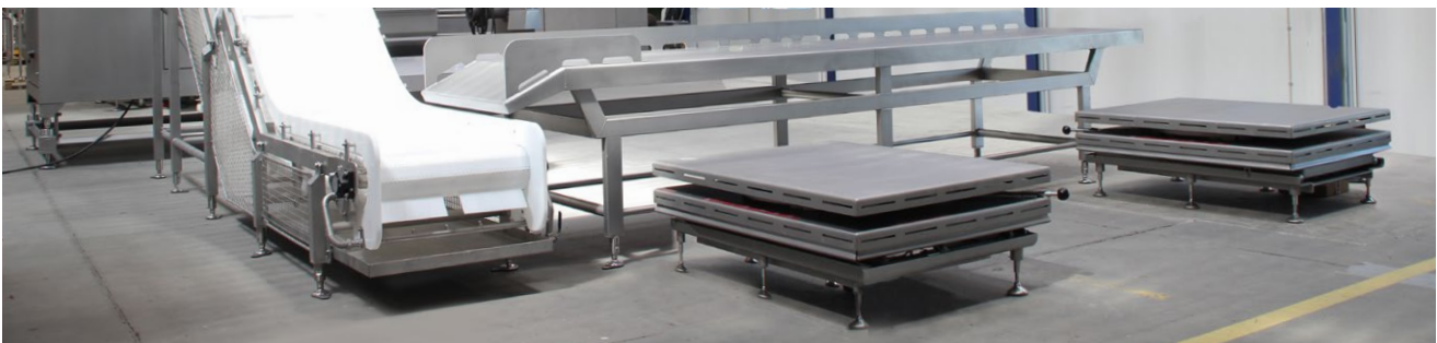
Belt Conveyor with unpacking station with 2 (two) lifting tables for ergonomics, left side.
