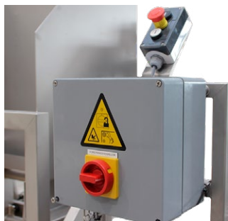
Operator/control panel with emergency stop.
