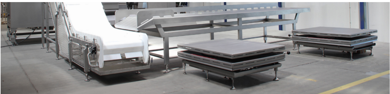
Belt Conveyor with unpacking station with 2 (two) lifting tables for ergonomics, left side.
