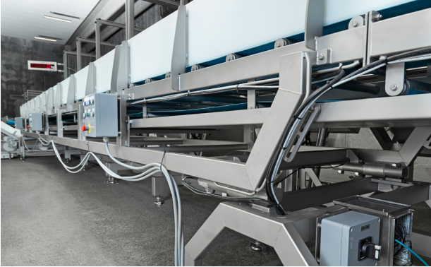
Belt conveyors with a range of standardized side rails and drip pans to avoid moisture and liquids on the floor.
