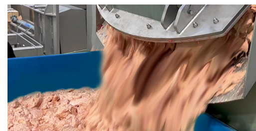
Cow udder product discharged from the scanDefrost.
