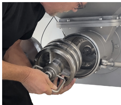
Assembly of the scanEmul 175 - Hopper fed knife cassette system. Quick and easy handling.
