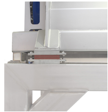
Bottom picture : Please note the shock absorbers which allow the WPC to remain stable (not moving) even when the WPC is fed by a fork lift truck dumping whole pallets into the crusher cabinet.
