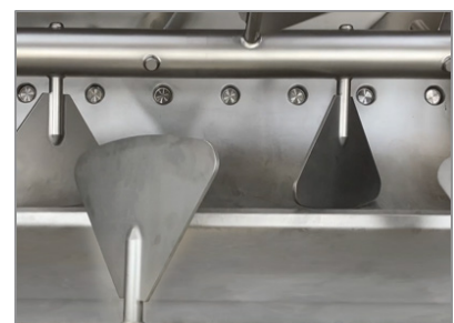
Paddle mixing wings, special application.
