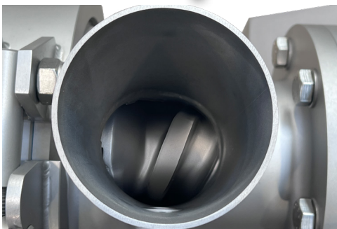
Top view of pump infeed section showing the worm/ auger of MC 250.
