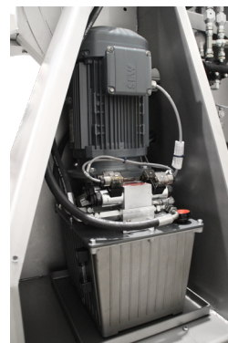
Pallet inverter seen from behind without cover, view of hydraulic unit and turning device.
