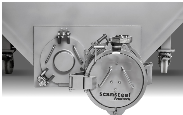
Shown above: Close-up of pump housing and side panel for second screw. Both designed for easy assembly/disassembly.
