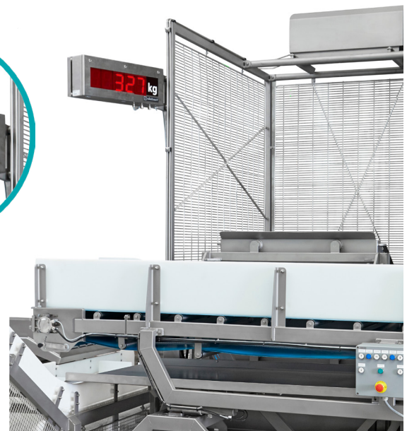
Details showing drip trays and weighing/load cells.
