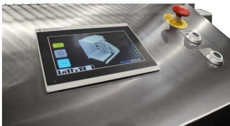
Electrical panel, including touch panel and manual buttons. The cabinet is certified stainless steel, AISI 304 execution.
